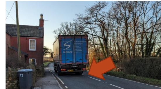
HGV passing through the gap. Note proximity of driver side wheels to central reservation.
